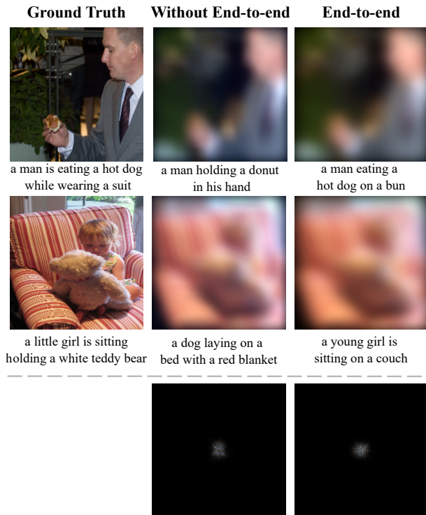
Fig. 4: Qualitative comparison of End-to-end vs. two-stage (without end-to-end) optimization approach. From left to right: Ground Truth, sensor image from the optical encoder optimized without end-to-end, and optical encoder trained end-to-end (ours). Below, the corresponding Point Spread Functions (PSF) are displayed for each approach.
